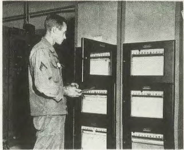
A Signal Corps technician checks the recording instruments where a continuous record of chain operation is plotted, enabling engineers to assess the operation of the system.
